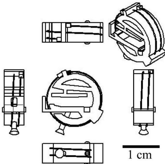
**S3.** Front, left, top, right, bottom and isometric views the shape memory alloy (SMA) wire actuated version of the peristaltic pump. SMA wire is shown wrapped around the pump body. A tensioning screw tensions the SMA wire around the body. Drawings to scale.
