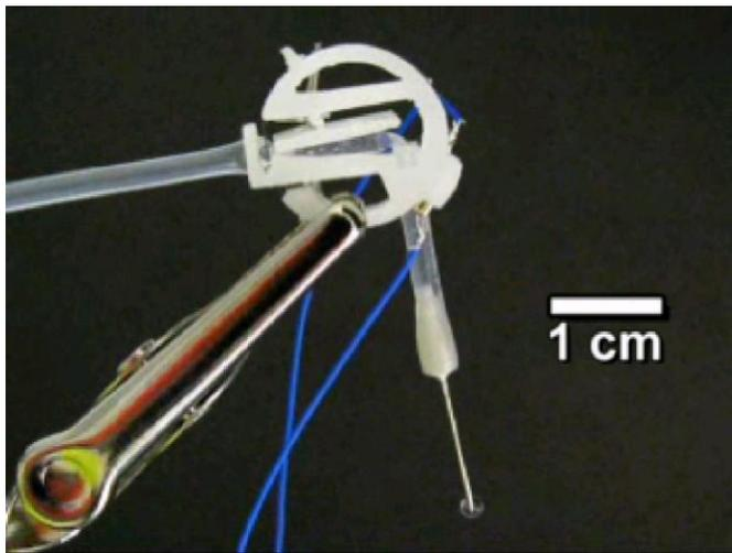
**S5.** Video of the SMA wire actuated version of the peristaltic pump (video uploaded as a separate file). This pump operates at 4 V, with minimal back pressure, pumping deionized water. Figures of merit for the pump: operating voltage, 4 V; flow rate range, 0 – 60  $\mu\text{l}/\text{min}$ ; operating pressure, 0 – 69 kPa; power consumption, 420 mW; weight, 0.9 g; package volume 1.3  $\text{cm}^3$ .
