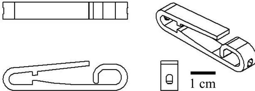
**S6.** Front, top, right, and isometric views (to scale) of the manually actuated version of the peristaltic pump. Drawings to scale.
