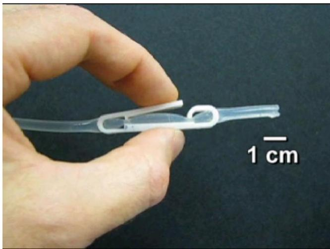
**S7.** Video of the manually actuated version of the peristaltic pump (video uploaded as a separate file). The pump is actuated by hand at several speeds and pumps deionized water with minimal back pressure. Faster actuation leads to larger flow rates. The pump weighs 2.6 g, and has a package volume of 4.2 cm<sup>3</sup>.
