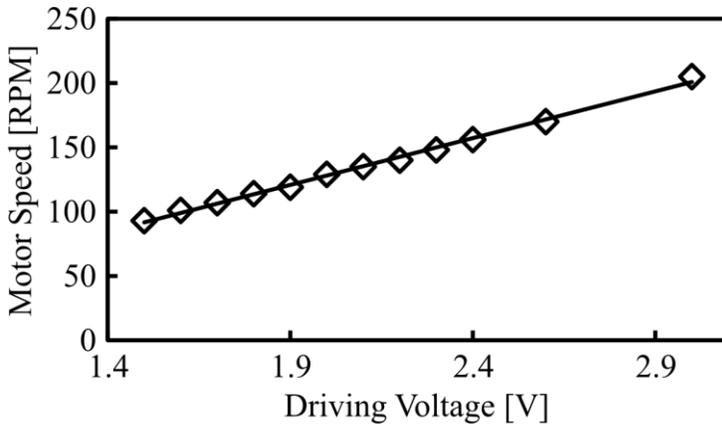
**S9.** Motor speed as a function of driving voltage while pumping deionized water at 22°C against minimal back pressure. As expected, motor speed (actuation frequency) increases linearly with driving voltage.
