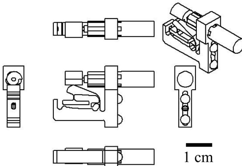
**S1.** Front, left, top, right, bottom and isometric views of the motor actuated version of the peristaltic pump. Drawings to scale.
