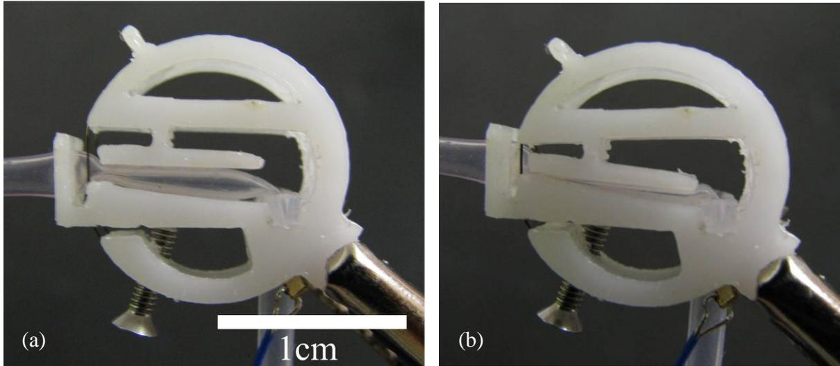
**S4.** (a) The SMA wire is relaxed (stretched): the upstream valve and pump chamber are both open and the pumping chamber refills from the upstream. (b) The SMA wire is contracted (electrical current is applied to the wire): the plunger closes the upstream valve and compresses the pumping chamber, raising the pressure within. This opens the downstream burst valve, and expels the fluid.
