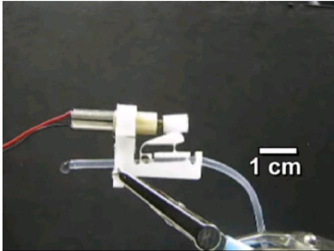
**S2.** Video of the motor actuated version of the peristaltic pump (video uploaded as a separate file). This pump operates at 3 V, with minimal back pressure, pumping deionized water. Figures of merit for the pump: operating voltage, 1.75 – 3 V; flow rate range, 0 – 780  $\mu\text{l}/\text{min}$ ; operating pressure 0 – 48 kPa; power consumption, 40 – 90 mW; weight, 3.6 g; package volume 6.2  $\text{cm}^3$ .
