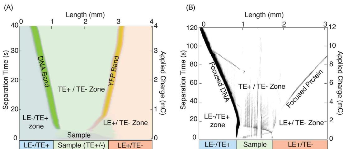
Figure S-3. Simulation and visualization of the dynamics of DNA and protein zones during bidirectional ITP process: A) Spatiotemporal representation of numerical simulation of ion concentrations during ITP. Each ion is given its own false color. B) Measured spatiotemporal plots determined from CCD images of protein and DNA zones focused in bidirectional ITP. Yellow fluorescent protein and DNA labeled with SYBR Green I were imaged using a custom fluorescence setup and a stereoscope.
