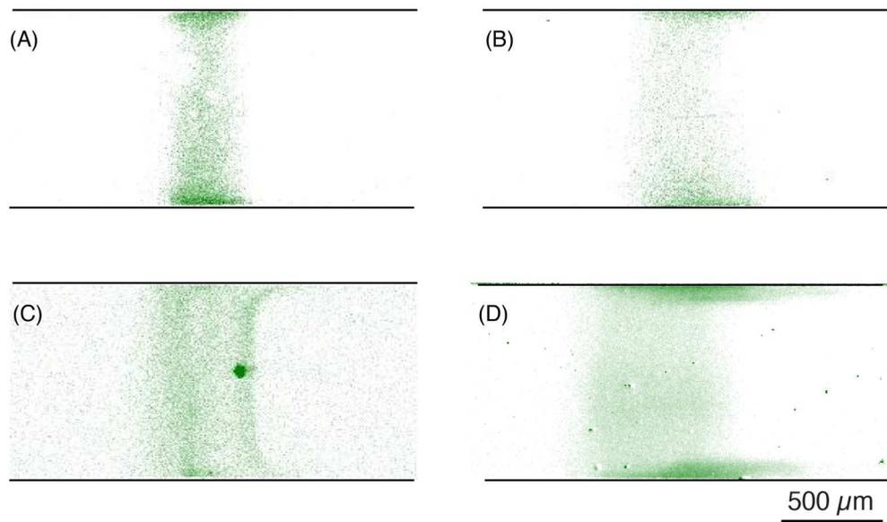
Figure S-5. Example images of fluorescence of DNA zones in ITP process from serum samples. (A)-(D) represent typical DNA zone shapes and fluorescence level in simultaneous extraction experiments where we spiked in salmon sperm DNA. We hypothesize nonspecific binding between DNA and serum proteins resulted in low collection efficiency for spiked DNA.
