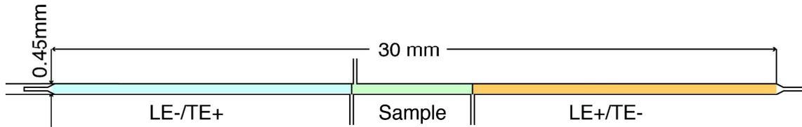
Figure S-4. Simple, straight channel design for visualization experiments. The main channel here was 0.45 mm wide and 30 mm long. Three side channels were used for loading buffers and samples. These also partition the main channel into three regions. We loaded samples to the middle region, LE-/TE+ buffer to the left region for DNA purification, and LE+/TE- buffer to the right region for protein extraction. The visualizations for this channel are shown in Figure S-3B.
