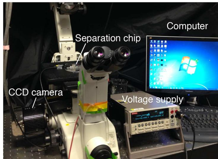
Figure S-2. Experimental setup. This set up includes an inverted epifluorescence microscope, a CCD camera, a voltage supply, and a computer for control of experiments and data acquisition.
