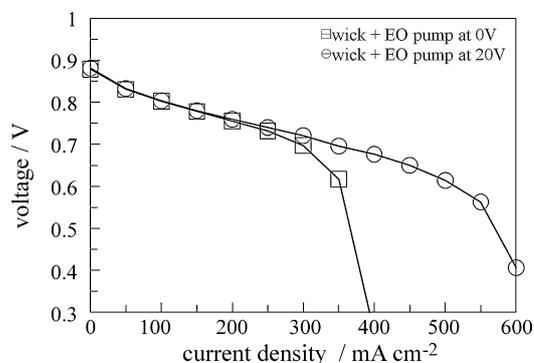
Fig. 3. Polarization scans of an EO-pump enabled air-breathing fuel cell with embedded wicking layer for EO-pump voltage settings of 0 V (pump off), and 20 V (pump on). The ambient conditions were 10 °C and 80% relative humidity and the conductive wick was 0.5 mm thick. Operation with a deactivated EO-pump leads to severe mass transport losses due to flooding. Activation of the EO-pump results in stable operation.
