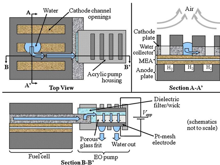
**Fig. 1.** Schematic cross-section view of an air-breathing cathode with an externally attached EO-pump hydraulically coupled to the fuel cell cathode via a porous, hydrophilic, thermally and electrically conductive wick ("water collector layer").
