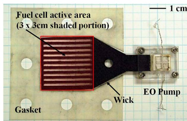
**Fig. 2.** Implementation of the wick layer with attached, external EO-pump. The wick layer area covers only the active cell area and is surrounded with a silicone gasket to minimize wick water uptake capacity and prevent gravity driven loss of water. The wick is patterned with parallel cutouts identical to the land areas of the cathode current collector.
