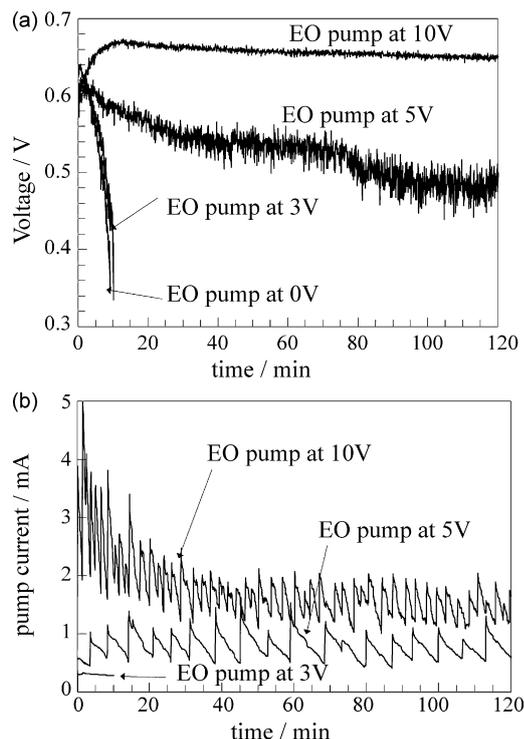
**Fig. 4.** Galvanostatic measurements of (a) fuel cell voltage and (b) EO-pump current in an EO-pump enabled air-breathing fuel cell with embedded wicking layer. The fuel cell was operated under flooding conditions  $T_{amb} = 10^{\circ}\text{C}$ ,  $RH_{amb} = 80\%$ , and  $j = 400\text{ mA cm}^{-2}$  for EO-pump voltages of 0, 3, 5 and 10V.
